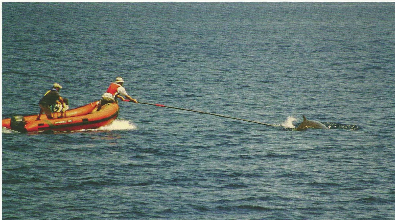
TAG TEAM—Researchers succeed in the challenging task of using a 40-foot carbon-fiber pole to attach a revolutionary digital recording tag, or D-tag, to an elusive whale during its brief stay at the surface between dives. The tag attaches with suction and records sounds and whale movements during several dives. It releases automatically after about 12 hours.
