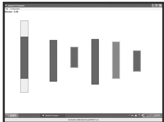
Figure 2. Graphical depiction of a PC-based tool for selection of frequency allocation tables. The vertical scale used for this graphical representation reflects distance along the cochlea. The range of the active frequency table is visually represented by a dark gray bar that is embedded within a larger, light gray bar (leftmost bar). The light gray bar represents the whole frequency range that is audible to humans. As the listener adjusts the frequency table, the dark gray bar moves and changes accordingly. Listeners modify the frequency map in real time until they find the one that sounds most intelligible. In addition to the continuous adjustment described above, the listener (or the experimenter) has the option of selecting a number of filter banks for further comparison. When a given filter bank is selected with the mouse, the corresponding dark rectangle is copied to the right of the screen (see five bars to the right of the figure). Any subset of those filter banks can be then selected for comparison. The active filter bank changes from one to the next, instantaneously, by pressing the space bar. During execution the program keeps track of which filter bank is active and saves the information to a file. Supplemental to the online version of this article is a version of this figure (Video 1) that demonstrates changes in speech intelligibility as the frequency table is adjusted while a talker speaks. Speech is initially unintelligible; it becomes better and becomes optimal as the frequency table moves up; and then it becomes unintelligible again as the frequency table moves even higher.
